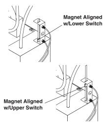
If the wash solution drops below the lower reed switch, the low water indicator light on the control panel turns on and the system disconnects power to the heating element, the pump, and the turntable motor. To reset the system, add water to the sump until the low water indicator light turns off.
