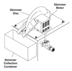
Allow the oil skimmer to operate until it is no longer extracting oil from the cleaning solution.
