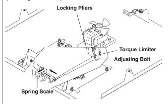
The torque arm should begin to slip at 7 pounds. If it slips at **less than** 7 pounds, tighten the adjusting bolt. If it slips at **greater than** 7 pounds, loosen the adjusting bolt.
